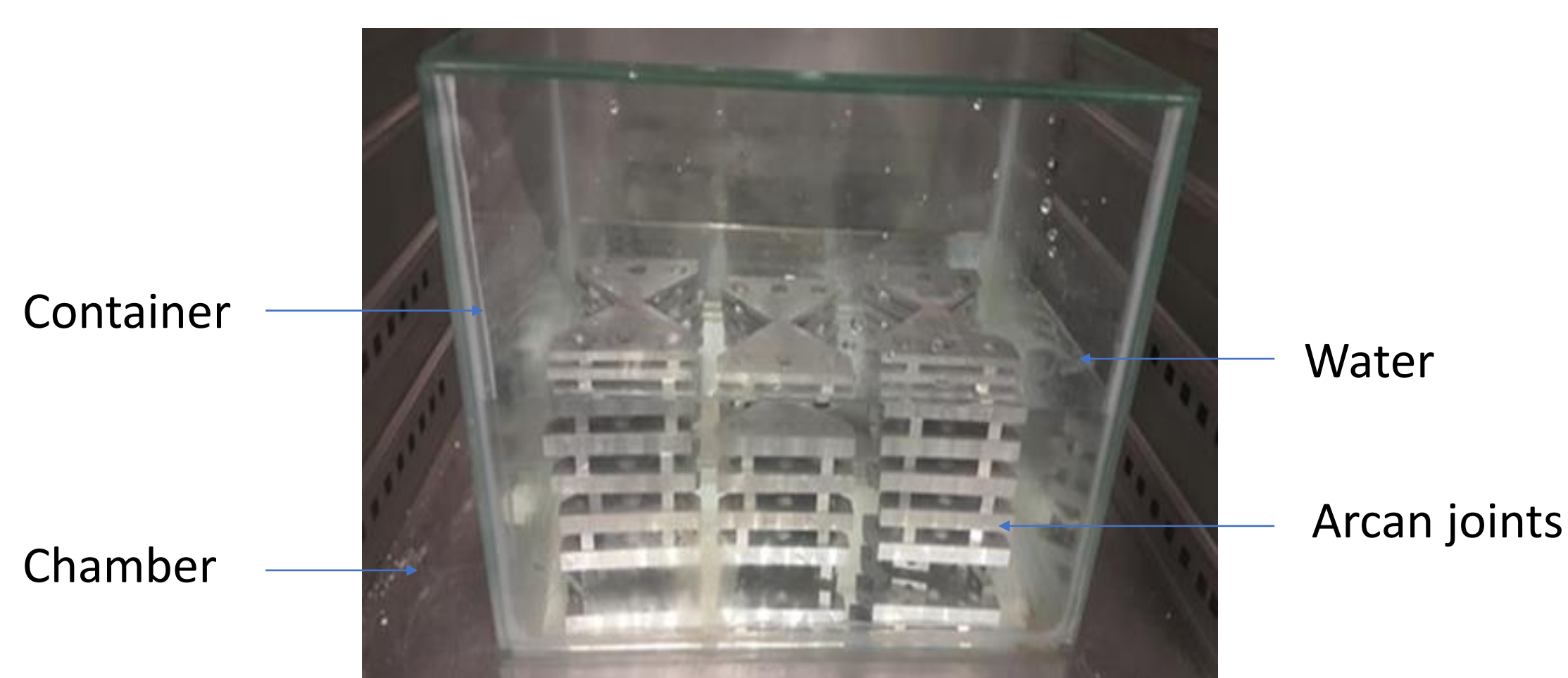
Figure 3 – Arcan joint ageing.
